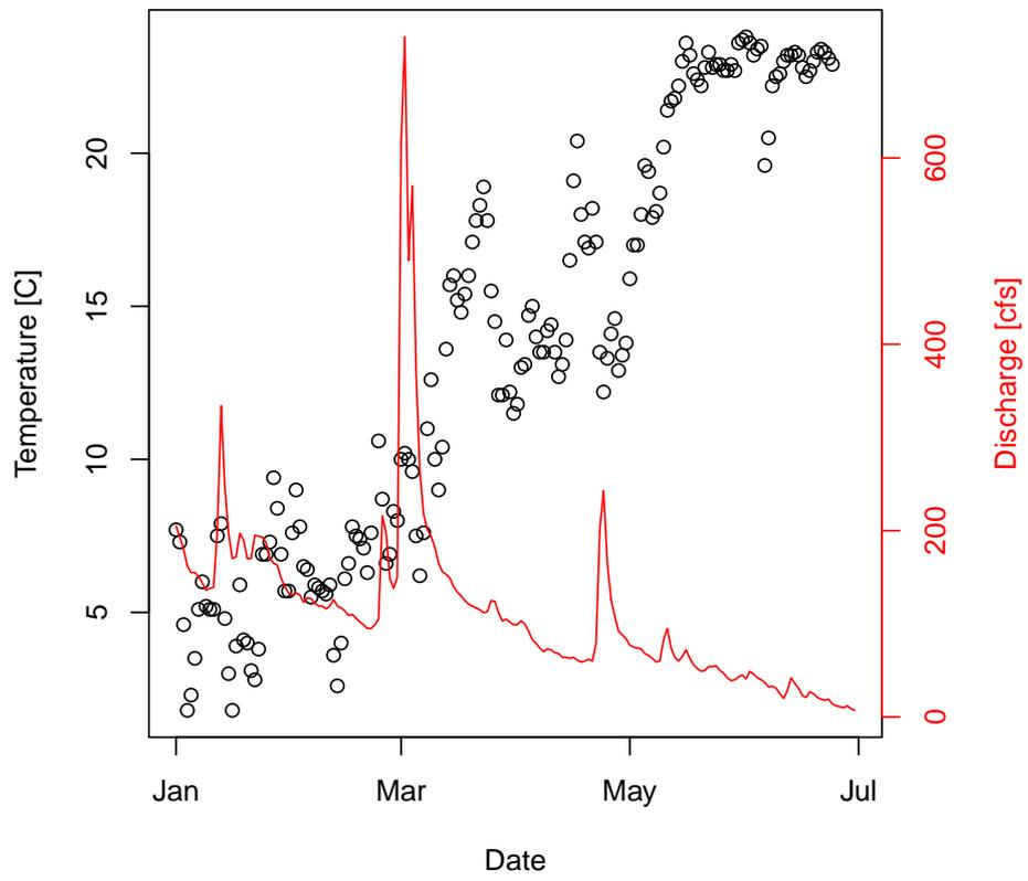
Figure 1: Temperature and discharge plot of Choptank River.
